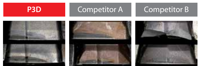
Wear comparison after drilling 48 holes
